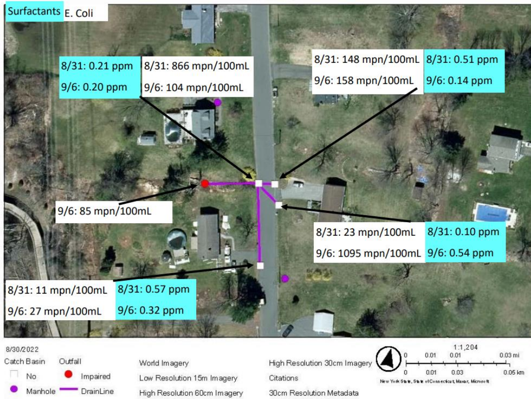
Figure 4: Trackdown Map on 4_Dean_OT1 and connected outfalls and storm drains. Surfactants data is in blue boxes and E. coli data is in white boxes. Red circle is the outfall. Squares represent storm grates. Purple circles are man hole covers. Purple lines show drainage connections.
